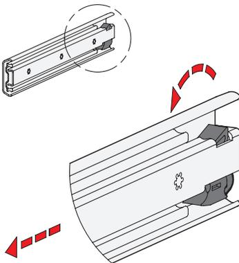
Telescopic slides GN 1422 have an integrated self-retracting mechanism, which improves considerably the ease of use when closing the extensions.
